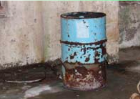
Full nitric acid drum discovered during inspection - note its state.
